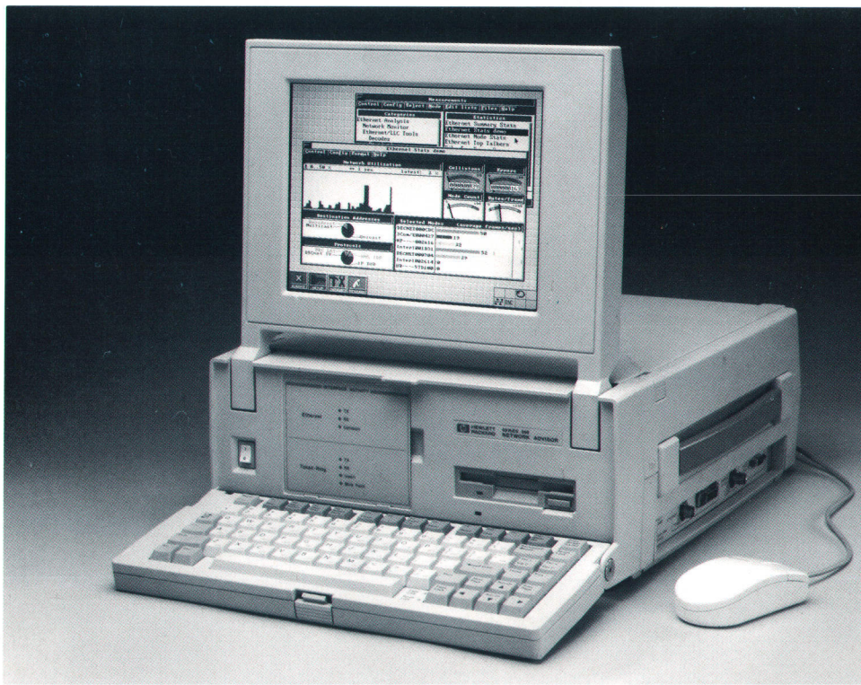
Fig. 1. The HP Network Advisor showing the mainframe and the folding keyboard and display. The display shows an example summary statistics screen in which graphical objects such as bar charts, pie charts, and gauges are used to present information.
